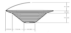
Figure 2. The Concept Prototype Model of the Innovative Device
