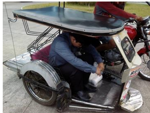
Figure 6a. Passenger experiencing a limited vertical clearance and backrest
