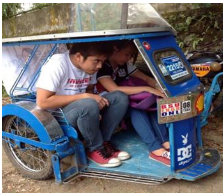
Figure 7a. Narrow passengers' seat for two passengers
