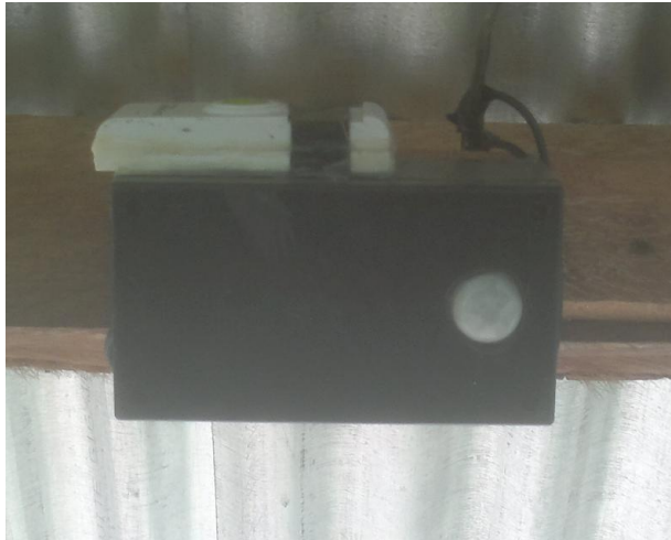
Fig.3 The modified body sensor and transmitter module. (The Circuit was adopted from Alexan)
