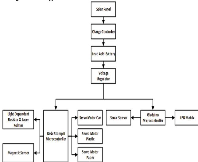
Fig. 1 Block Diagram of Solar Powered Electronic Trash Can
