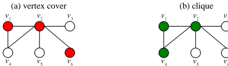
Figure 2. Given an example graph G = (\{v_1, v_2, \dots, v_6\}, \{(v_1, v_4), (v_1, v_2), (v_2, v_4), (v_2, v_5), (v_2, v_3), (v_2, v_6)\}) , then (a) a vertex cover C of G with k = 3 are the red-colored vertices, while (b) a clique of G with k = 3 are the green-colored vertices.
